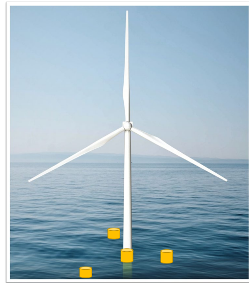
Figure 1. IFE-UTD-NTNU 25 MW Wind Turbine on Semi-submersible Floater
