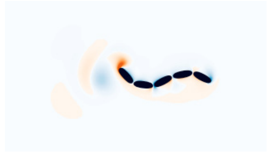
Fig. 3. Snapshot of the swimmer in the high-fidelity simulation, showing vorticity in a clockwise direction (red) and counter-clockwise direction (blue).
