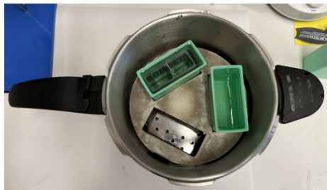
Figure 2. Set-up of the ITO slides inside of the pressure cooker.
