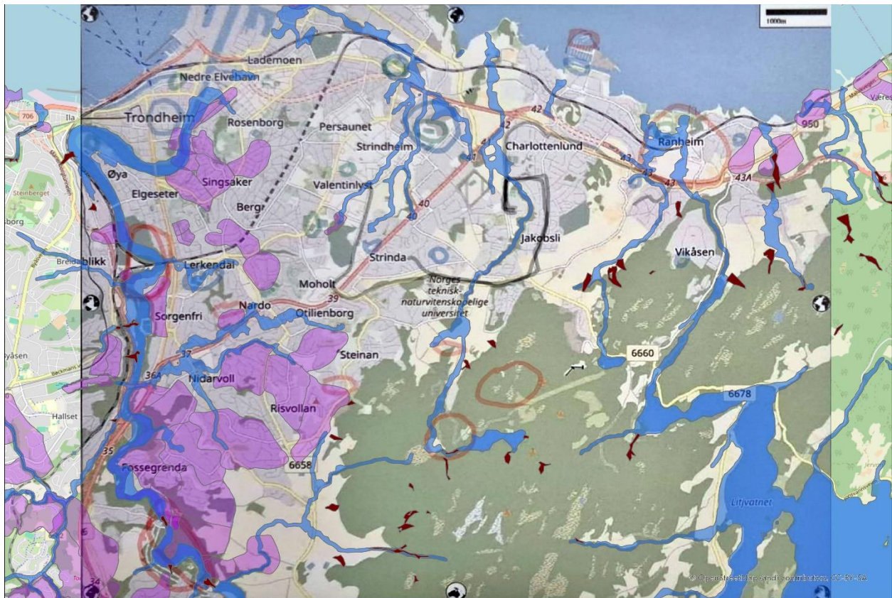
Figure 37 - Map 17 to 19 displayed with the natural hazard layers, where purple represent quick clay, translucent blue represent flood, and the dark red areas represent landslides, from (NVE, 2024). Picture exported from ArcGIS Pro (esri.com, 2024).
