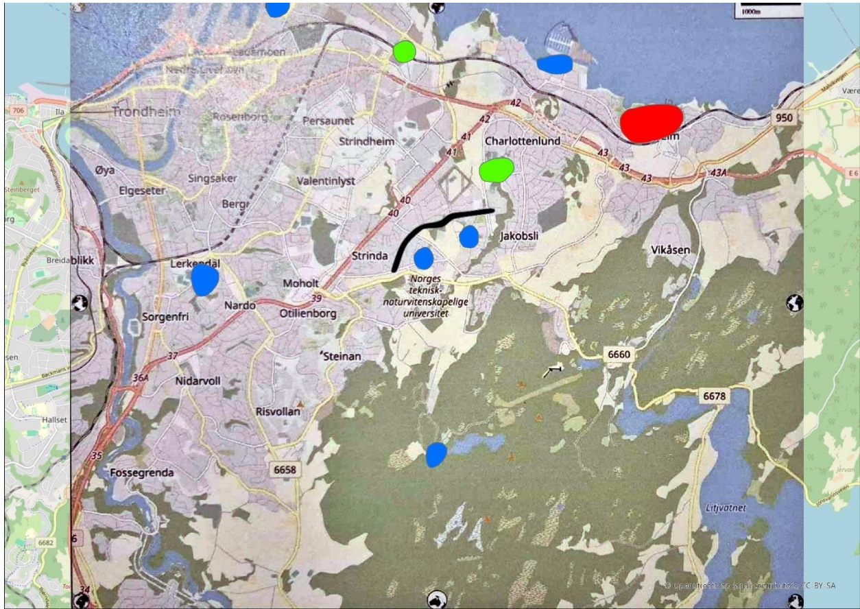
Figure 15 - The GeoTIFF result for map 8 after correcting the symbology for polygon 3 and 9. The raster for map 8 is used as the background. Picture taken in ArcGIS Pro (esri.com, 2024).
