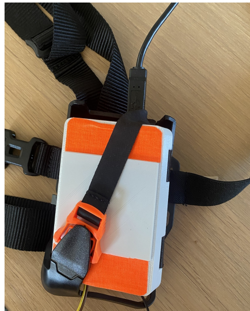
(b) Printed case for Arduino and IMU with mounting strap.
