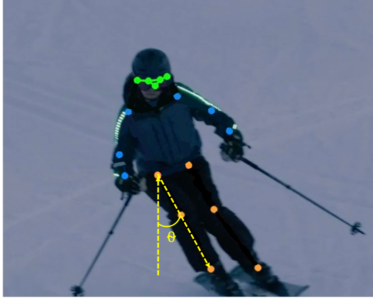
Figure 17: Skier with keypoints and vectors used for calculating angle with respect to vertical.
