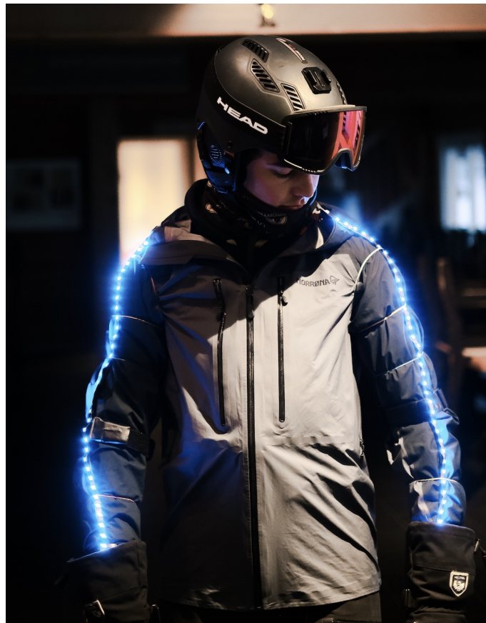
Figure 8: LED system mounted on skier. The LED strips stretch from the shoulders to the wrists, and the rest of the system is covered by the skier's jacket.
