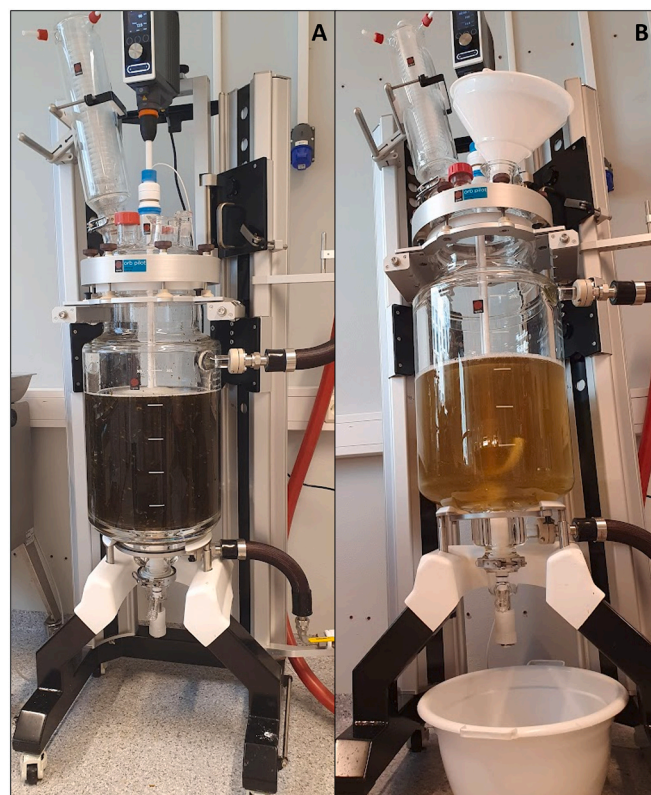
Fig. 7. Upscaled in-process epimerisation on SL -biomass in PilotOrb. A) Milled Saccharina latissima -biomass in 21 L of ion-free water with pH adjusted to 7 (after acid wash of biomass), and B) Extracted alginate solution added AlgE1.
