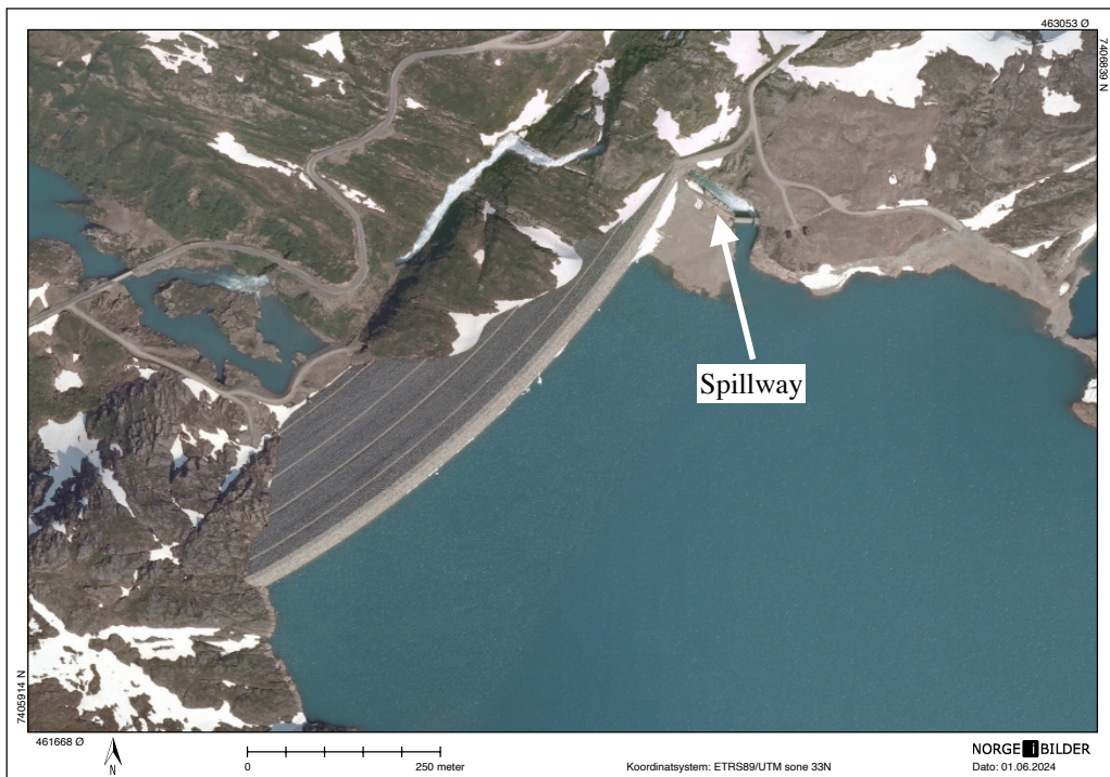
Figure 4.43 Aerial photo of Storglomvatn dam on the eastern side of Storglomvatn, with large concrete dam spillway visibly active at northern end. Photo from NorgeiBilder.no (Norge digitalt, 2024).
