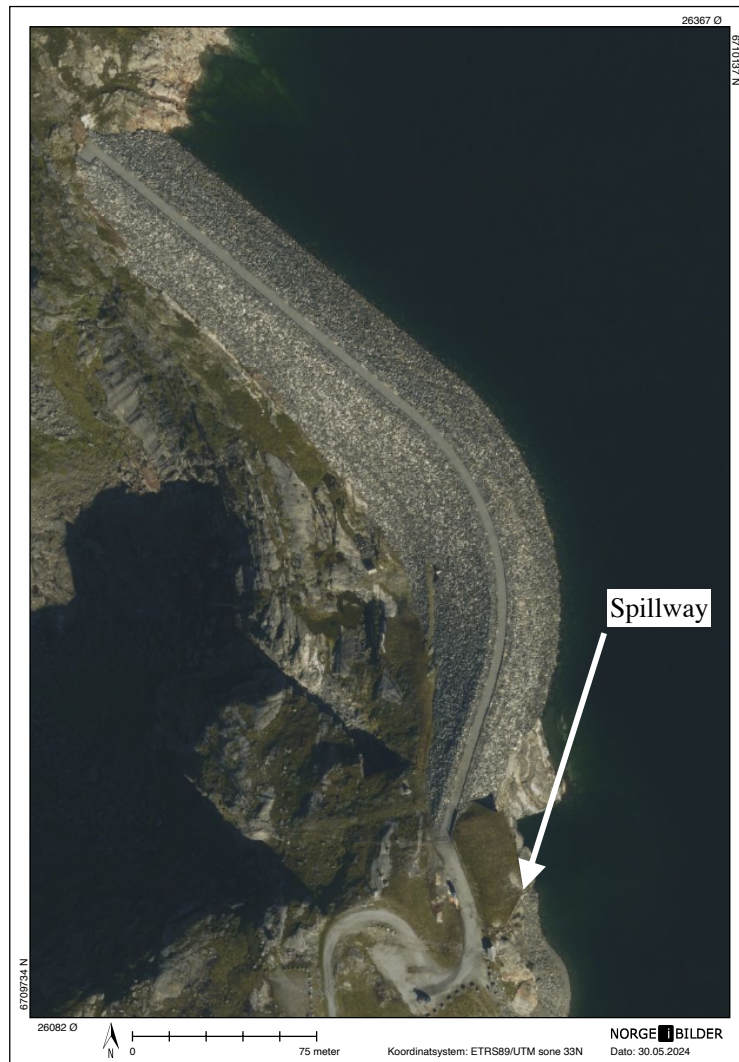
Figure 4.20 Aerial photo of Dravladalsvatn dam, with spillway structure visible out south end, leading to a flood channel underneath the road. Sourced from NorgeiBilder.no (Norge digitalt, 2024).
