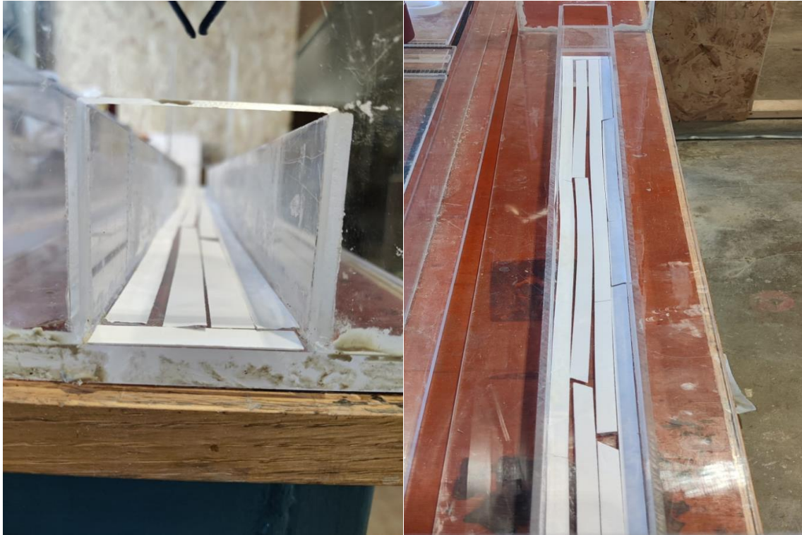
Figure 17 Double-sided tapes placed on the invert
