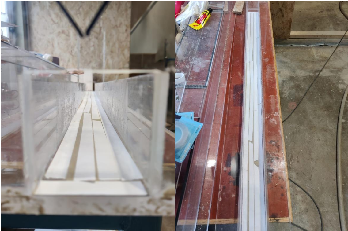
Figure 18 Water sealant clay between gaps of tapes
