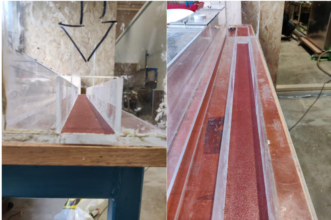
Figure 20 Placement of sandpaper over the invert
