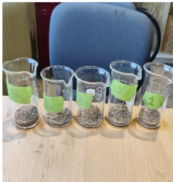
Figure 26 Glass containers used for sand injection
