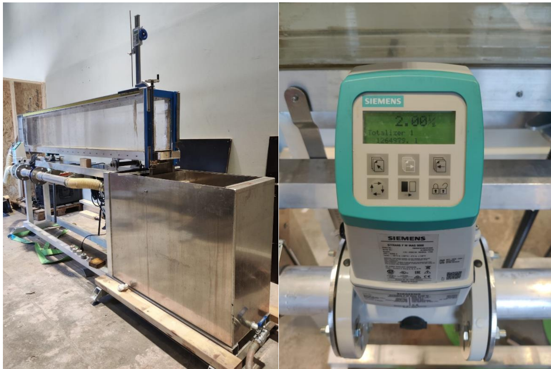
Figure 9 Mini flume - Test rig on the left and digital flow meter on the right
