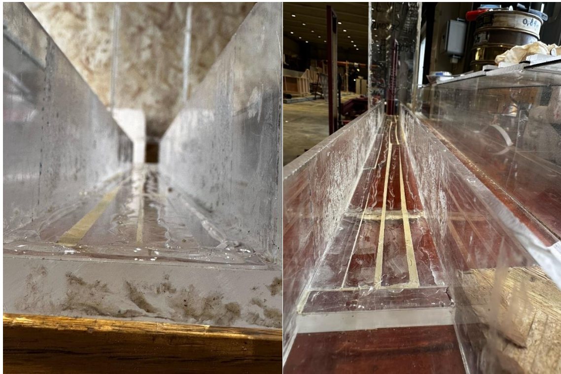
Figure 19 Application of super glue over double-sided tapes
