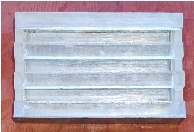
Figure 13 Sandbox of model 100-A with ribs
