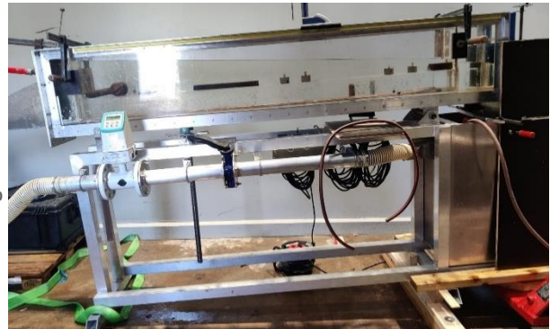
Figure 22 Model with the slope of 4° inclination
