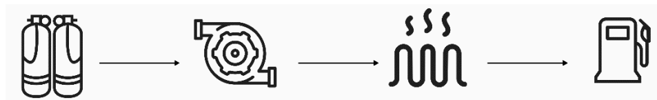
Figure 3.9 Schematic Diagram for HRS with Liquid hydrogen in tanks
