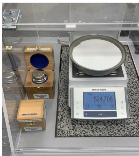
Figure 5. Set-up of test procedure of a specimen on the high-precision balance
