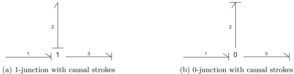
Figure 11: The common flow and effort junctions with assigned causality and numbered power bonds.
