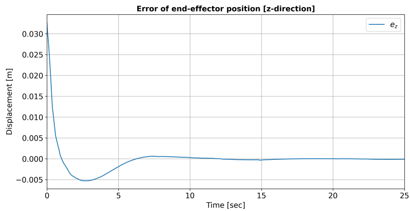
Figure 70: Here e_z is the error between the desired and measured crane tip position in z -direction.
