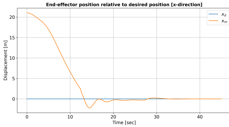
Figure 85: x_d and x_m is the desired and measured end-effector position in x-direction
