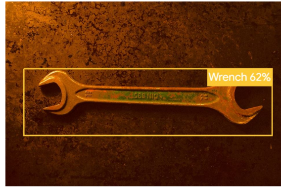
Figure 6.29: Correct wrench prediction with 62% confidence score. The prediction score threshold was set to 25%.
