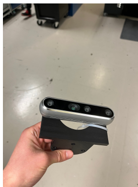
Figure 5.2: Intel RealSense D455 camera mounted on the bracket used to attach it to the robot end-effector.
