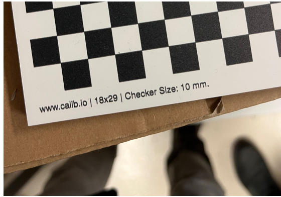
Figure 5.8: Dimensions of the chessboard pattern. The image was captured using a mobile phone camera.
