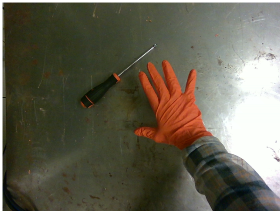
Figure 6.3: Failed hand detection when wearing orange gloves and holding no items. A screwdriver was present on the work table.
