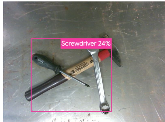
Figure 6.36: One single screwdriver prediction, placed on the pile of objects with an acceptable level of precision. The hammer and wrench went undetected. The prediction score threshold was set to 15%, and the bounding box predictions were made using MediaPipe Studio.
