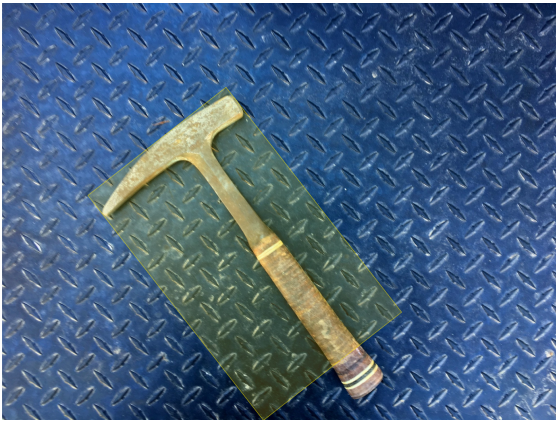
Figure 6.22: Bounding box placed parallel to the handle, arguably representing the natural and intuitive orientation. The bounding box reached the edge of the image and did not encapsulate the entire hammer.
