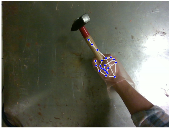
Figure 6.8: Successful hand detection when wearing a transparent glove and holding a hammer. However, the index finger landmarks were out of position.
