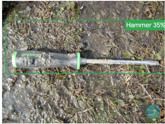
Figure 6.26: Screwdriver wrongfully predicted as a hammer with a 35% confidence score. The prediction score threshold was set to 25%. Image source: Eugene Peretz via Flickr, license: CC BY-SA 2.0 DEED. Bounding box prediction was made using MediaPipe Studio.
