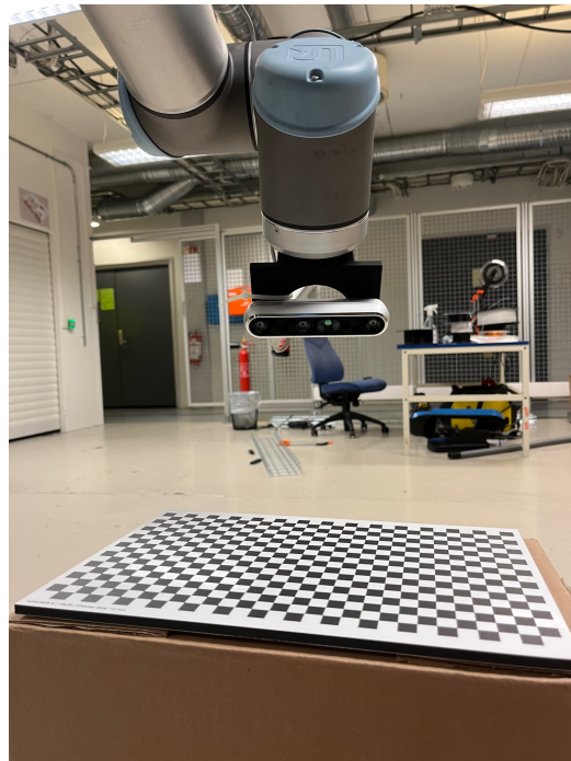
Figure 5.10: Close-up image of the Intel RealSense D455 camera and the chessboard pattern while recording images for the camera calibration procedure.
