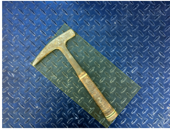
Figure 6.23: Bounding box tilted compared to the handle, allowing the entire hammer to be encapsulated while keeping the bounding box as small as possible. This example represents a possible ambiguity in the labeling process.
