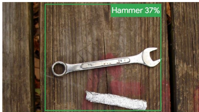
Figure 6.27: A wrench wrongfully predicted as a hammer with a 37% confidence score. The prediction score threshold was set to 25%. Image source: Kevin via Flickr, license: CC BY-NC-SA 2.0 DEED. Bounding box prediction was made using MediaPipe Studio.
