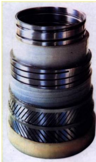
Figure 11: Typical flexible pipe cross section (Sævik 2017).
