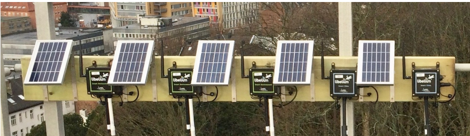
Figure C.12: Testbed with five of the eight sensor nodes
