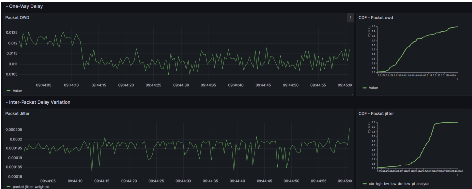
Figure 4.6: A screenshot from the detailed dashboard showing the visualizations for the OWD and the IPDV.
