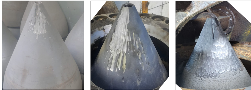
Figure 2: Stages of erosion on a coated needle, HPP at Ancash, Peru.
