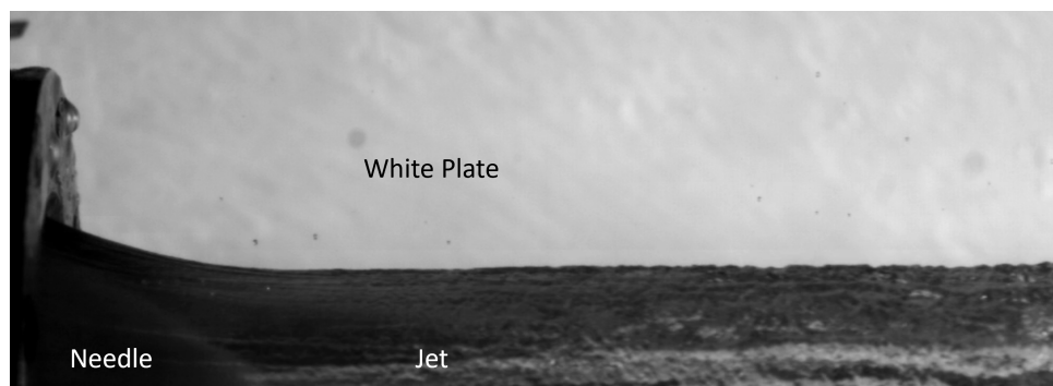
Figure 7: Camera image captured at a shutter speed of 1/400000 seconds to delineate the jet's border along the flow direction
