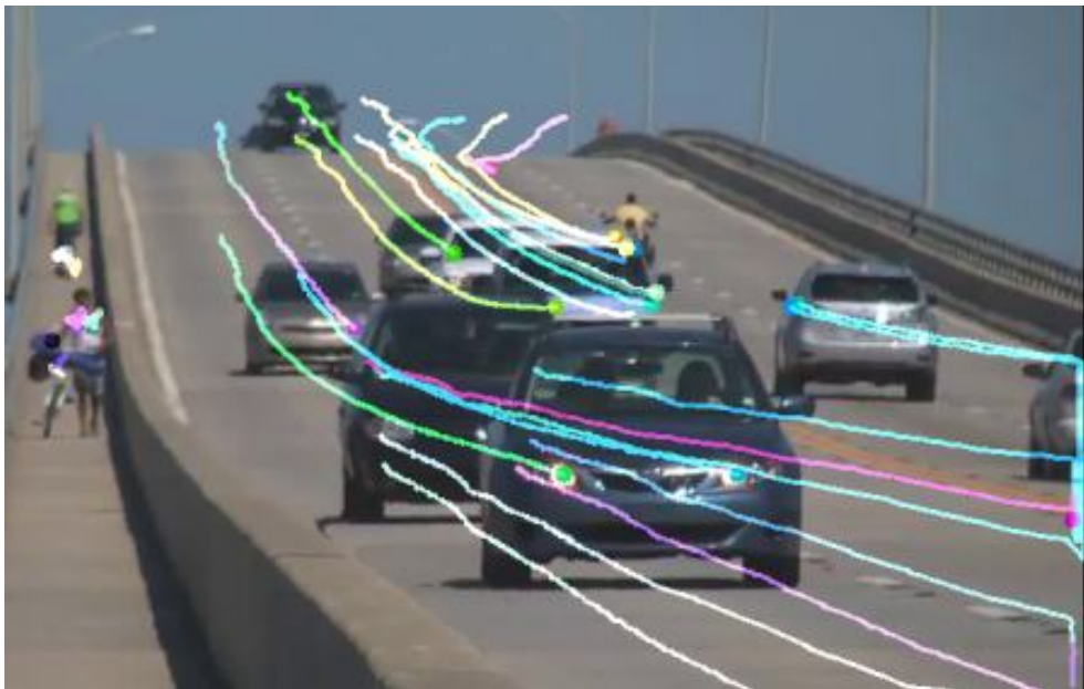
Figure 4.8: Demonstration of optical flow tracking, from [63].
