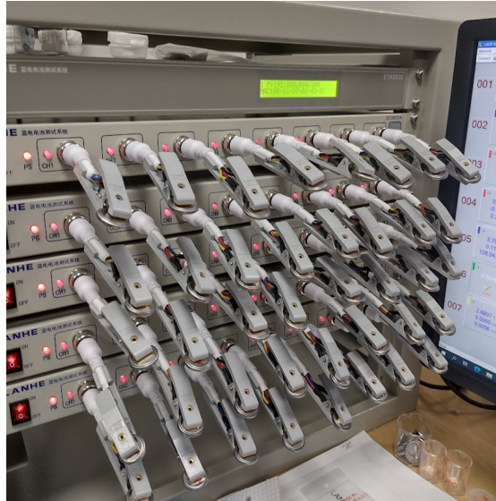
Figure 3.3.1: This is a picture showing the LanheCT3002A - Land Battery testing system & data processing software used for cycling the coin cells
