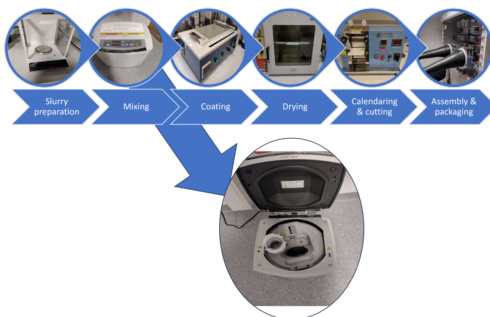
Figure 3.2.3: This is a figure showing the mixing equipment for a Lithium-ion battery in a lab. The slurry is placed inside the "cupholder" which is then secured in the larger "cubby".
