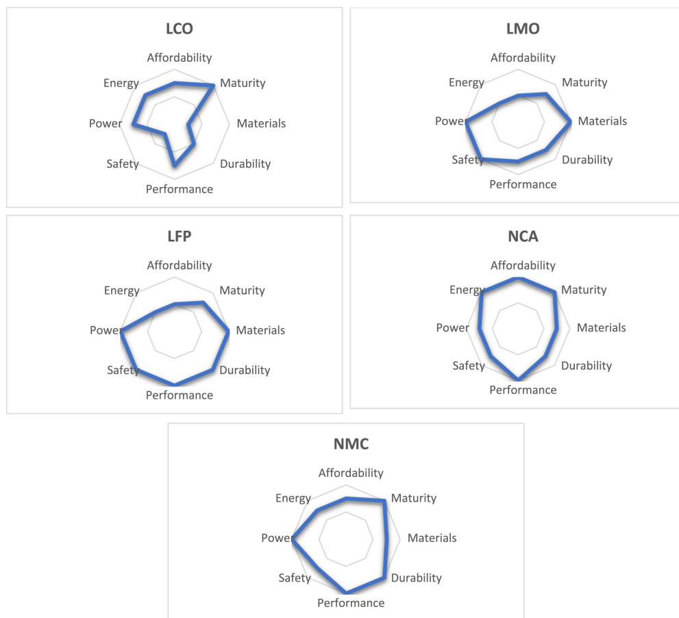
Figure 2.1.6: This is a figure showing the strengths of the main cathode chemistries and compared against each other. Figure taken from Zubi et al.[21]
