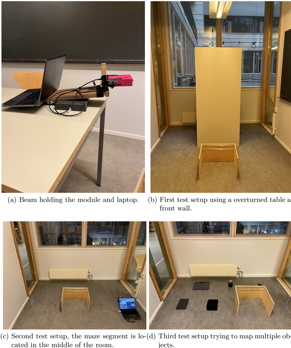
Figure 6.9: Test setups where the position estimate is used as position reference when creating a map of the room.
