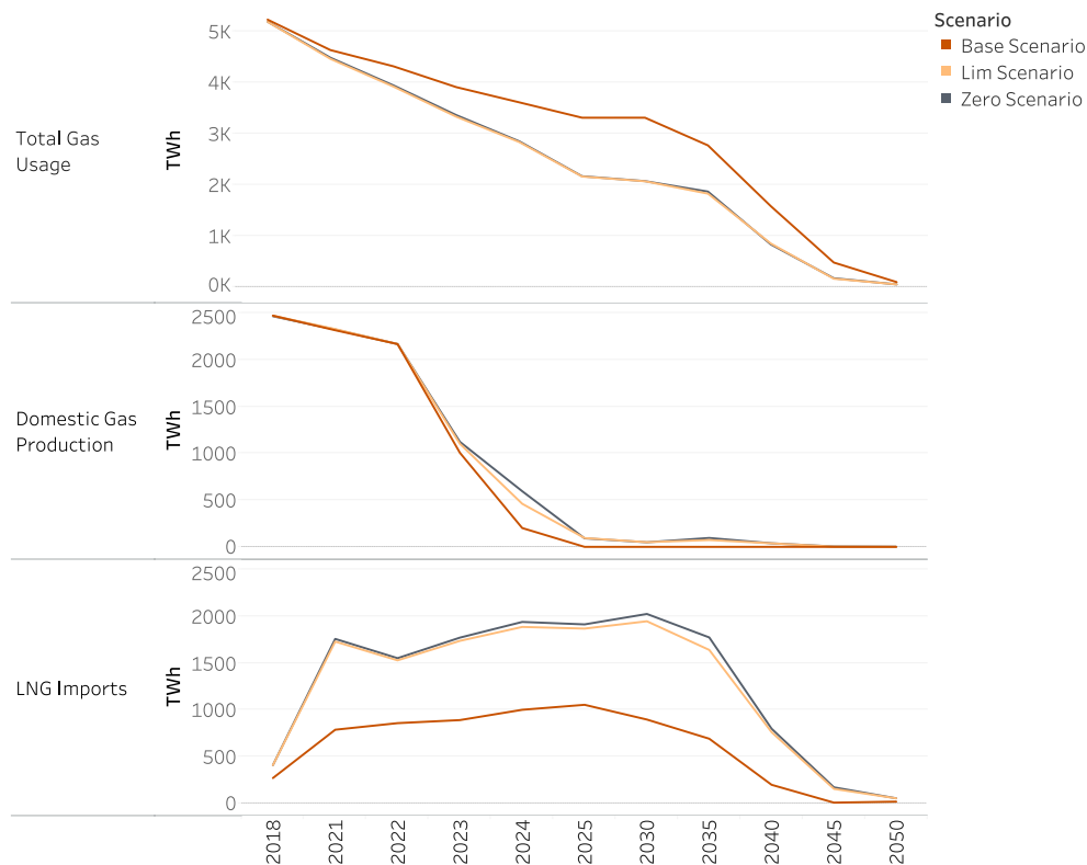
Fig. 4. Results for total European gas use (top), domestic (European) gas production (middle), and LNG imports (bottom) until 2050, considering a 2 °C target. Source: Own illustration.
