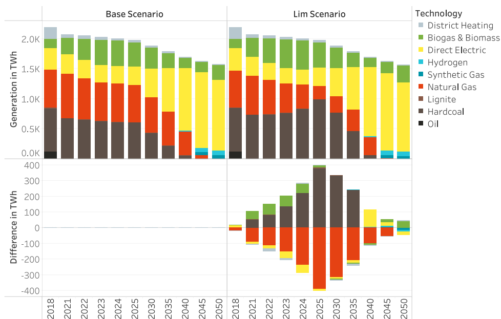
Fig. 7. Development of process heat generation in industry (top) and difference to the Base scenario (bottom) in Europe until 2050. Source: Own illustration.
