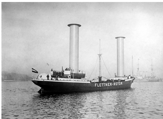
Figure 3.2: Magnus effect on a rotor sail generating a lift force acting perpendicular to the inflow. Figure courtesy to Korei (2017).
