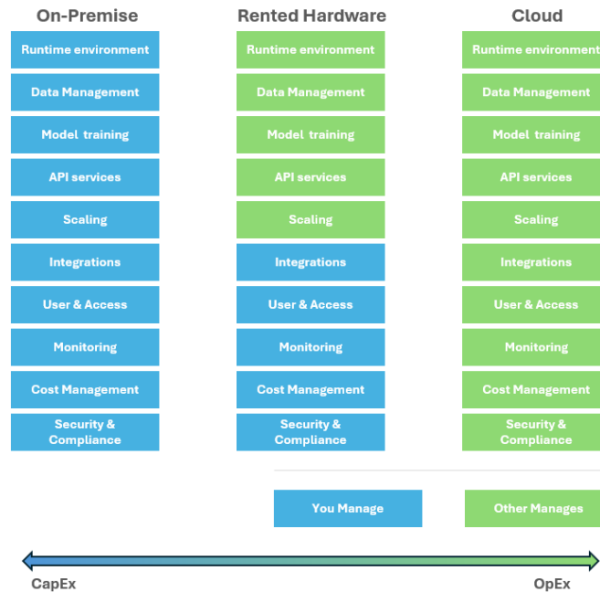
Figure 4.1: An overview of delivery methods for large language models and each method's respective area of responsibility.
