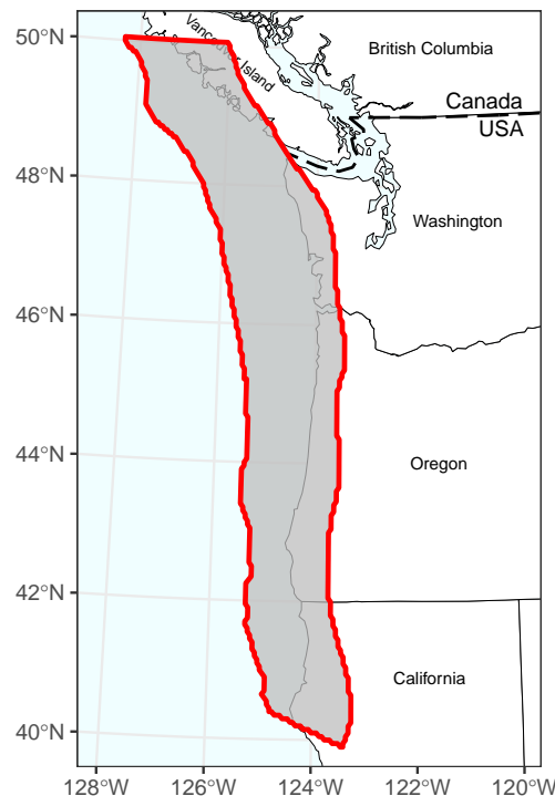
Figure 1.0.1: The area in grey, bounded by red, is the CSZ fault region which will be considered throughout this study. It was created by bounding the point depths of the Slab2 data set [25] which are less than 30 km deep.
