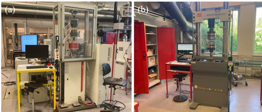
Figure 19: StepLab – Multiaxial 20 kN (a) and MTS 809 Axial/Torsional Test System (b) fatigue testing machines.
