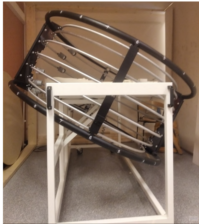
fig. 54. Heliodon set to the latitude of Trondheim, limiting the access to the table
