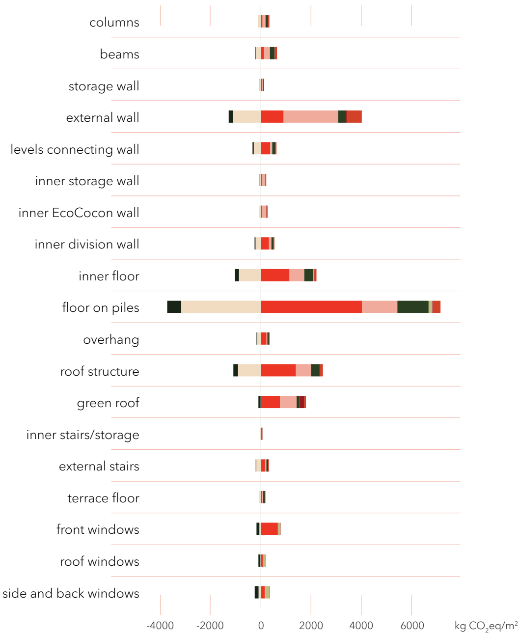
Fig. 38 Green roof cabin emissions by elements
