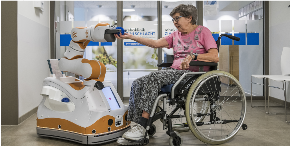
Figure 1.1: The service robot, Lio, interacting with a nursing home resident. Image source: (F&P Robotics AG, 2022)
