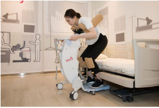
(a) A demonstration of the lifting robot, Hug, assisting in lifting a person from the bed. Image source: (FUJI CORPORATION, 2024)
