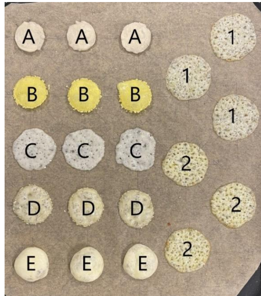
Figure 9. Melted samples from Schreiber test after 5 minutes in 200 °C oven, with Sample A (cashew), B, C, D, E (starch), 1 and 2 (dairy) (Figure 4)
