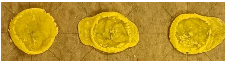
Figure 11. Triplicate of samples B (starch) after 12,5 minutes in a 200 °C conventional oven. The uneven spread is attributed to breaches in the dry crust, which caused liquid PBCA within to pour out.
