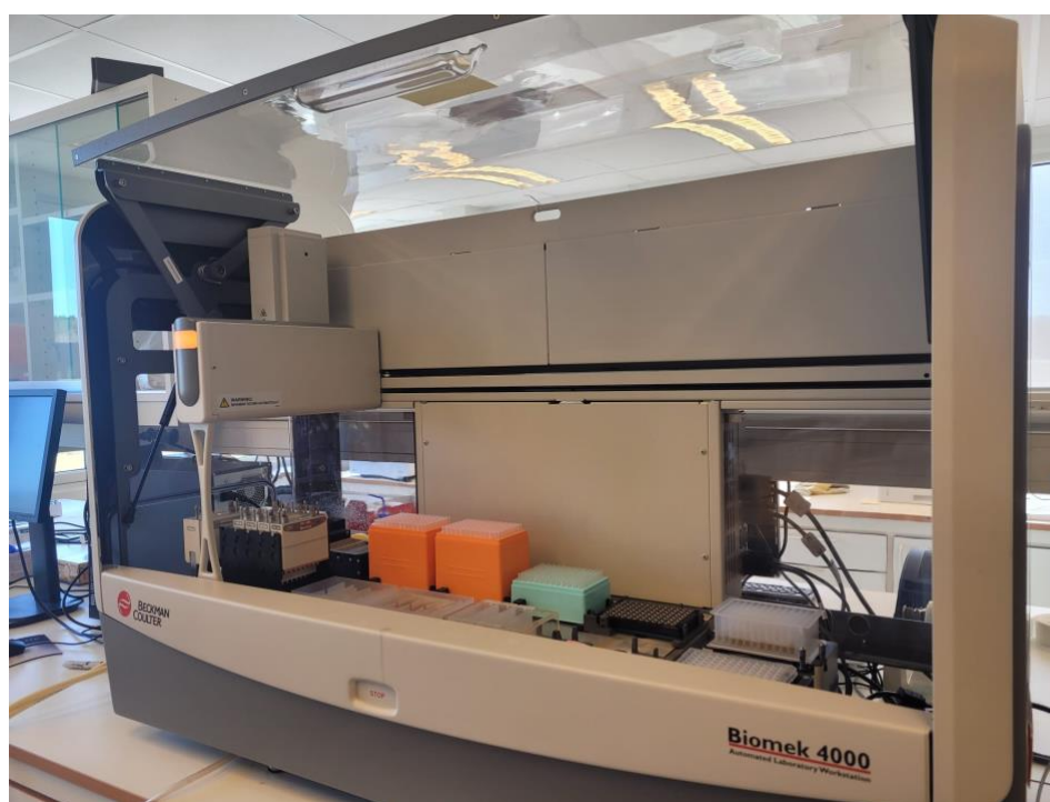
Figure 4. Biomek 4000 robot used for the extraction of RNA.
