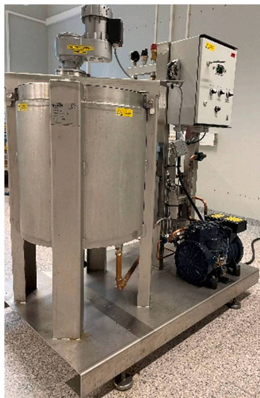
Fig. 1. Processing tank used for the sequential extractions: 100 L AISI 904L stainless steel tank, with two bladed stirrer and heating mantle, custom built by Skala Fabrik, Norway.
