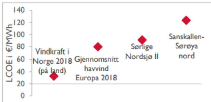
Figure 2.1: Comparison between Norwegian offshore wind prices and the rest of Europe by the Norwegian water resource and energy directorate(NVE) [9].
