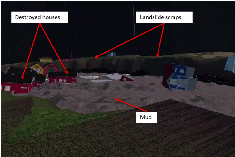
Fig. 6 Post-failure events showing the quick clay “mud,” slide scraps and destroyed houses
