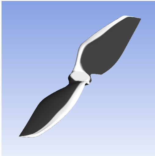
Figure 12: Ice shape of the 15-inch rotor at -10^{\circ}\text{C} obtained from a 3D ice accretion simulation.
