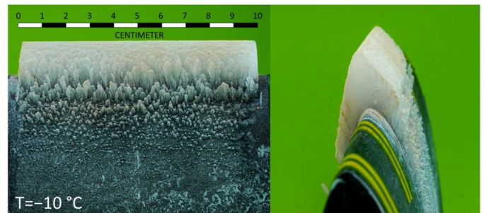
Figure 11. Close-up photo of the rime ice shape.
