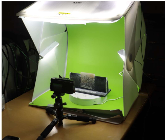
Figure 8. The photogrammetry setup with the removable leading edge situated on top of the turntable, inside the light box. A camera on a tripod is taking a series of pictures as the turntable rotates the ice shape.
