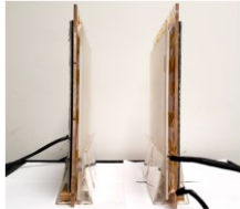
Fig. 7. A photo of IPT coils used in the experiment.
