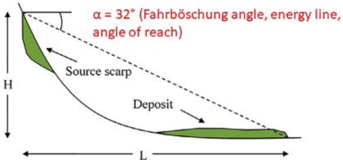
Figure 1: A schematic drawing representing a rock avalanche with Fahrböschung ( \alpha ), fall height ( H ) and run-out length ( L ). Modified from: Hermanns et al. (2022)
