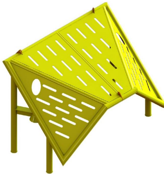
Figure 7: NL Project Sealine Protection Cover (SPC) [10].
