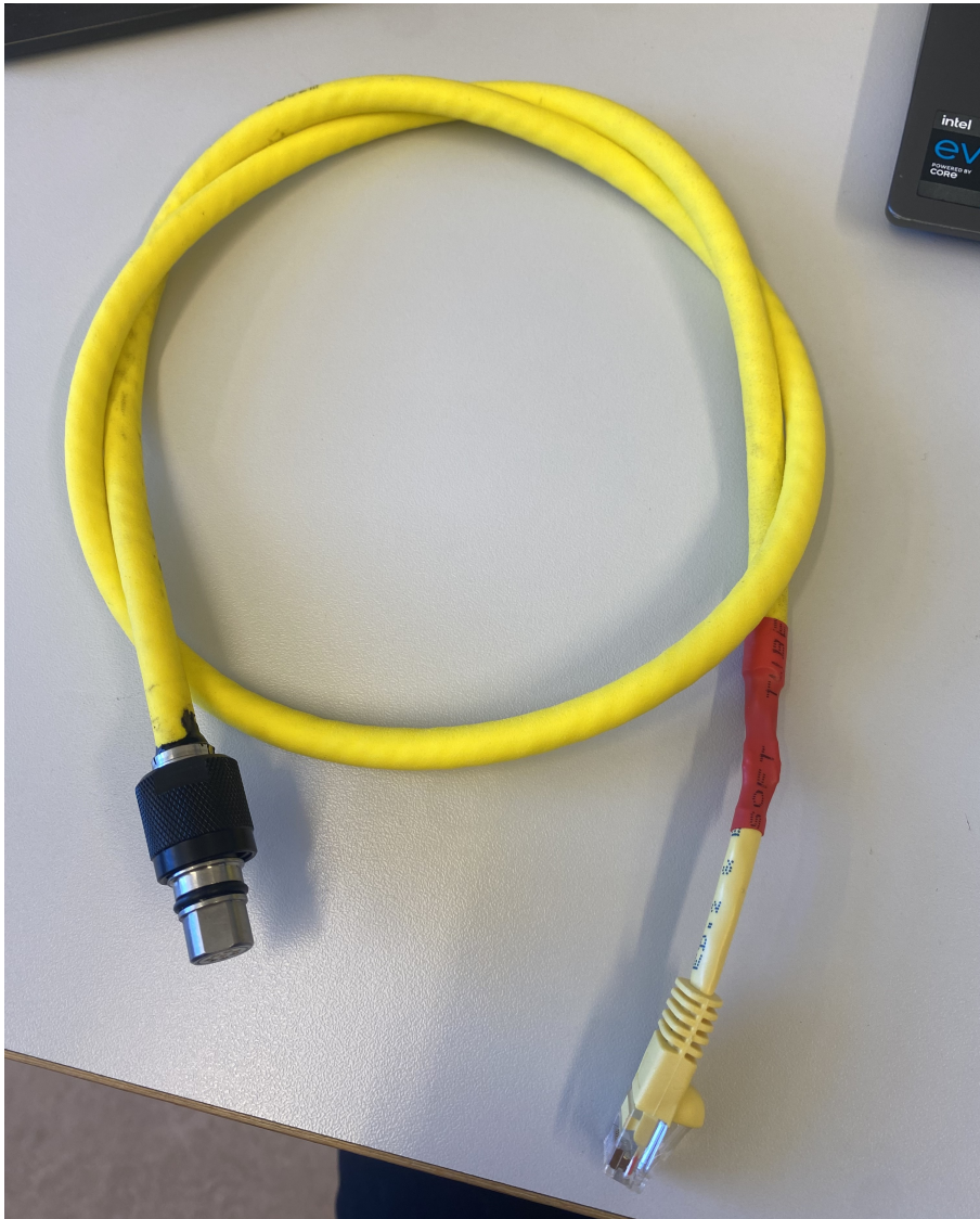
Figure 29: Cable for Ethernet Connection
