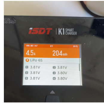
(c) Battery Cell Voltage
