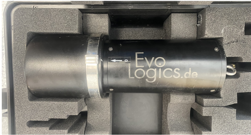
Figure 17: EvoLogics' Acoustic Modem
