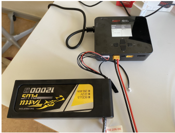
(a) Connection between Battery and charger
