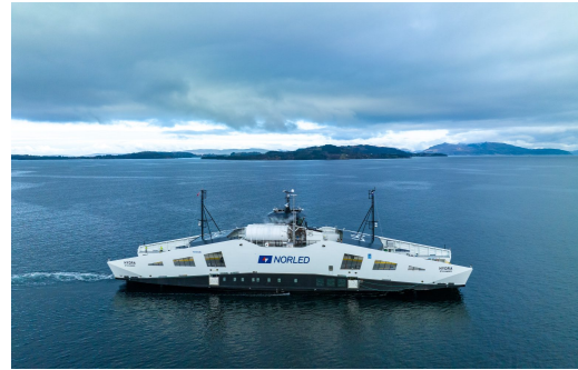
(b) The worlds first ferry driven partly on H_2 , MF Hydra [81]
