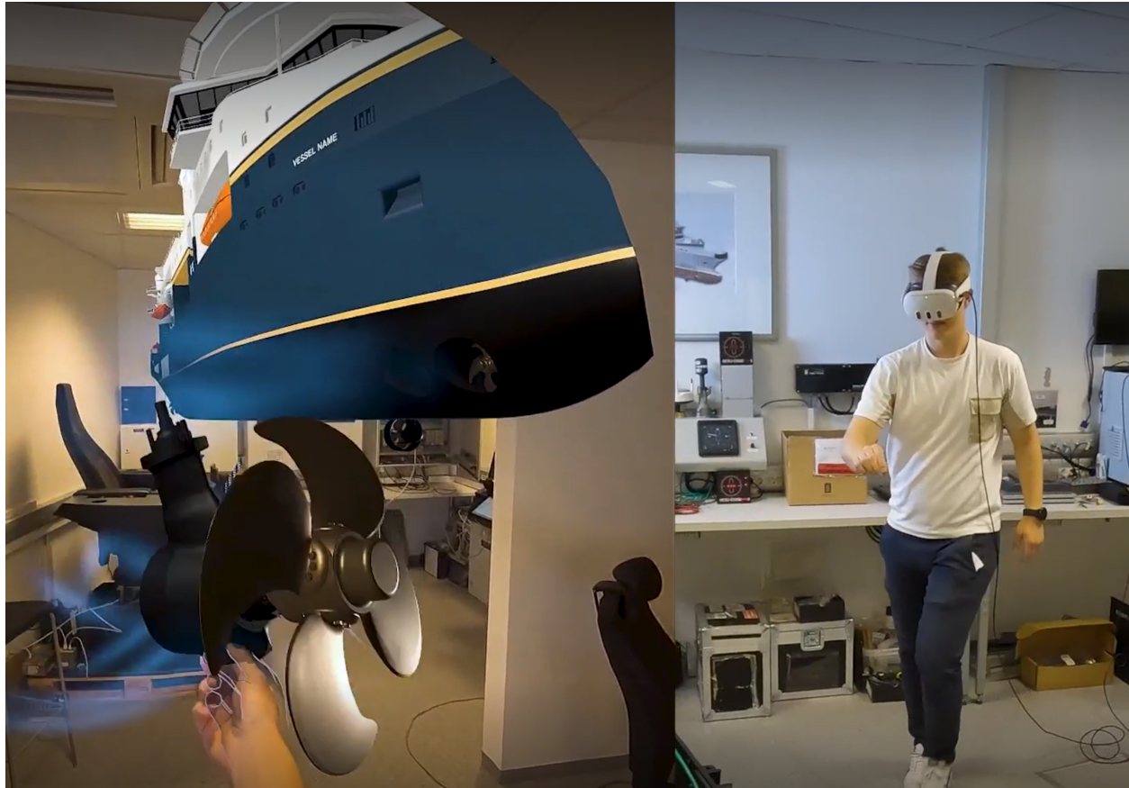
Figure 47: AR Visualization of Thrusters in Action: Real-time displaying active thrusters controlled by a system, complete with dynamic thrust direction indicators.
