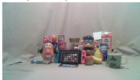
(d) Image after correction. Colour temperature setting 1 and brightness 100%.
