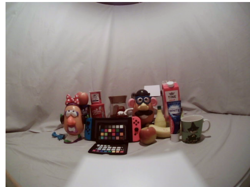
(d) Image after correction. Colour temperature setting 1 and brightness 100%.
