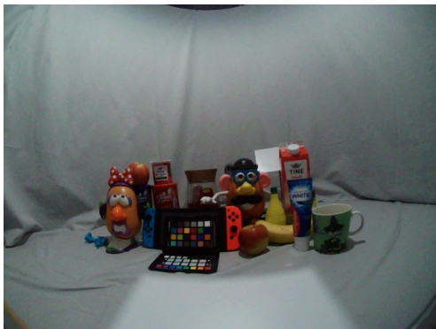
(e) Image before correction. Colour temperature setting 6 and brightness 10%.
