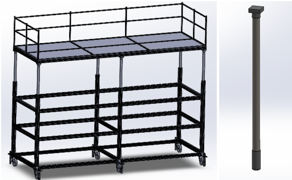
Figure 64: Simplified version of the platform featuring six columns and steel tubes, with POM safety components.
