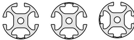
Figure 79: Some of the different groove-options from item24's website [65].
