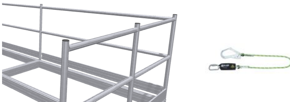
Figure 38: The designed railing and an example clamp-on [67] that can be used as anchorage.
