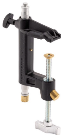
Figure 84: "Quick-Release Clamp" where the screw can be moved without needing to rotate it when the gold button is pushed in, but otherwise works as a regular screw [68].
