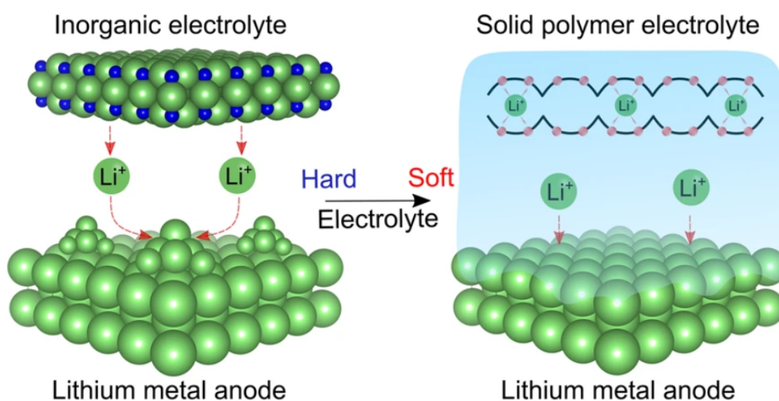
Figure 2.43: Comparison of ISEs and SPEs in LMBs. Reprinted from Song et al. [193]
