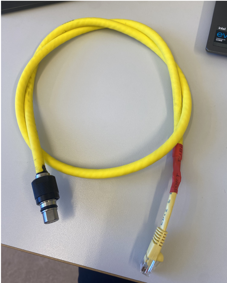
Figure 29: Cable for Ethernet Connection
