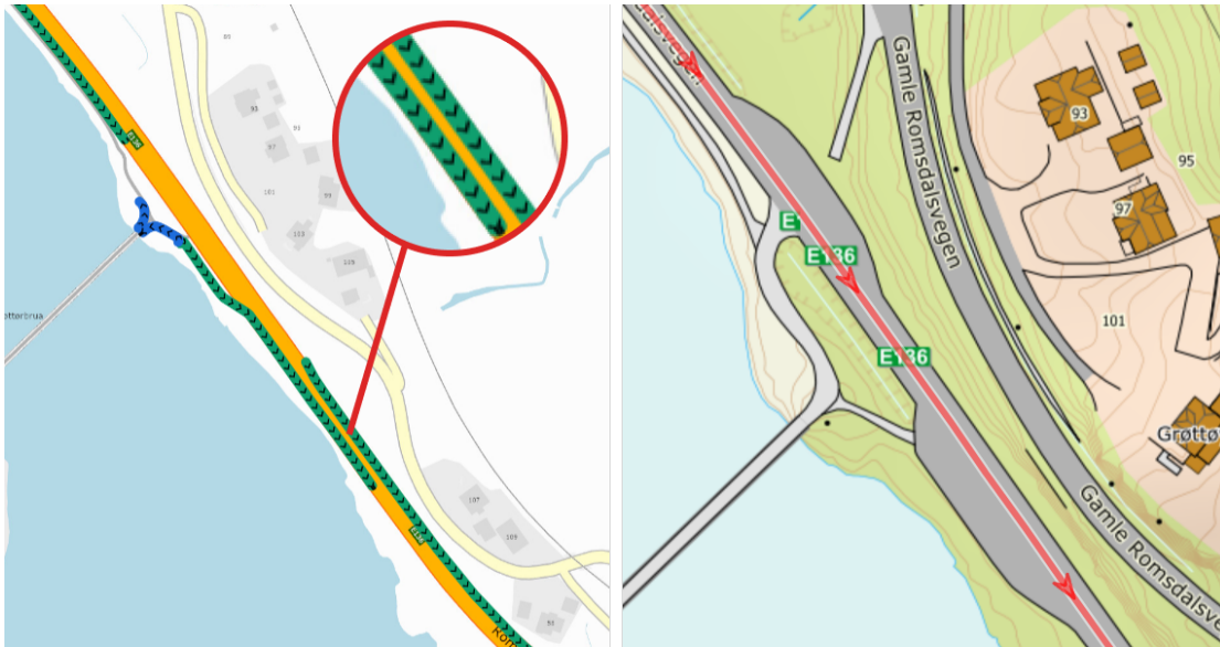
Figure 4.4.9: Comparison of railing geometry directions with road network direction
