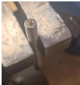
Figure 18: Magnet integrert i skulderaksel
