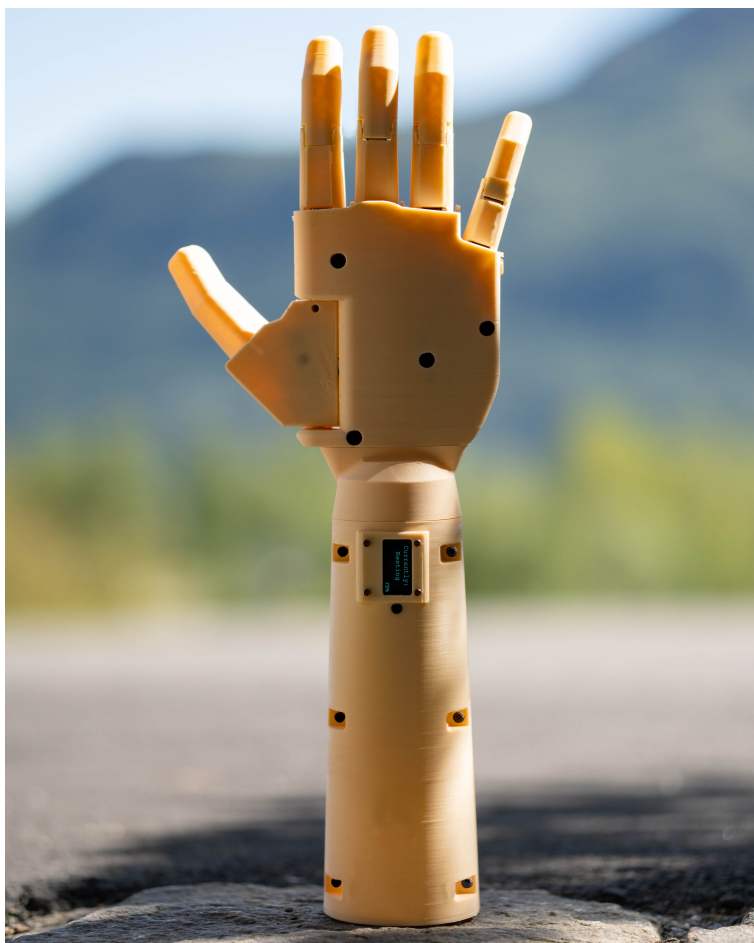
Figure 4.1: Final prototype of prosthesis powered on in resting position
