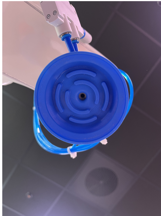
Figure 14: Gripper with hard contactpoints built inside the vacuum chamber
