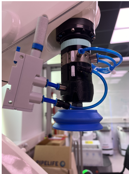
Figure 35: The chosen suction cup
