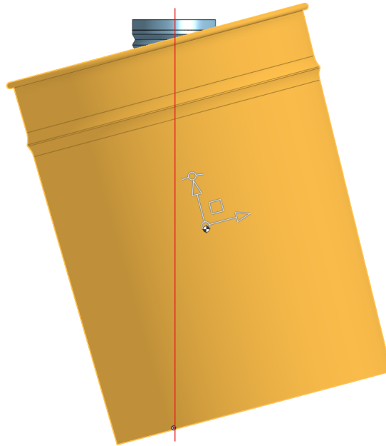
Figure 12: Representation of centre of mass under movement due to inertia and sloshing
