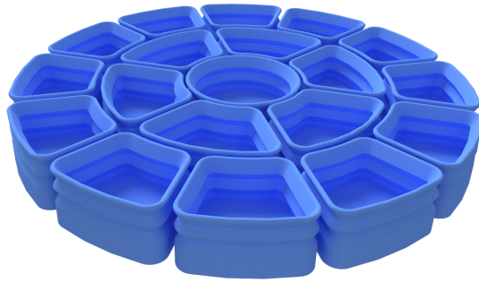
Figure 13: Gripper with compartmentalized suction cup
