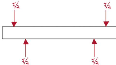
Figure 5.2.1: Free body diagram that shows the forces working on the test piece, with the exception of the force from the normal load given from the friction ball.
