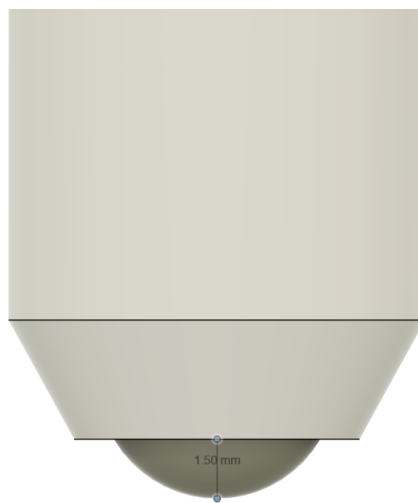
(c) Length of the alumina ball protrusion at 1.50 mm.
