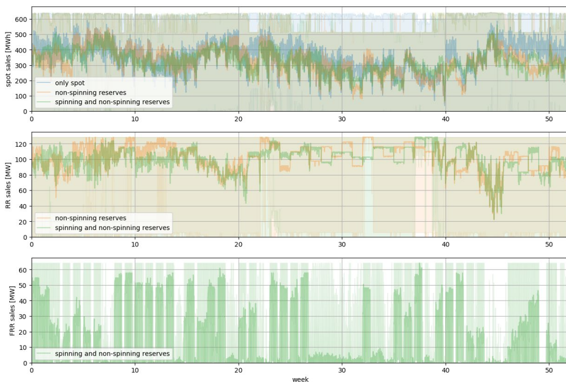
Figure 16. The energy sold on the spot market (top), non-spinning reserve market (middle), and spinning reserve market (bottom). Each panel shows the averages as solid lines and the minimum to maximum range as a semi-transparent area. All results are from SHOP.
